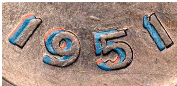
1951 Romania 2 Lei where the doubled die has been shaded blue and the mechanical doubling has been shaded red
