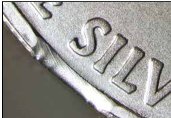
Reverse with clip (left) and corresponding area of weakness opposite the clip (right).
