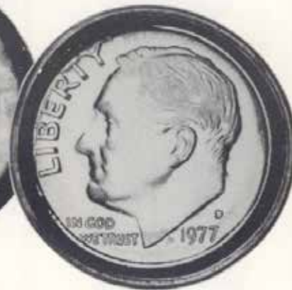
1977D Roosevelt Dime. Deep capped die piece. Large distorted brockage on reverse — date shows. BU $375.00
